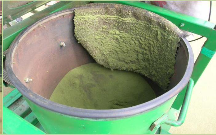
Contamination that has been extracted from astro turf court infill
