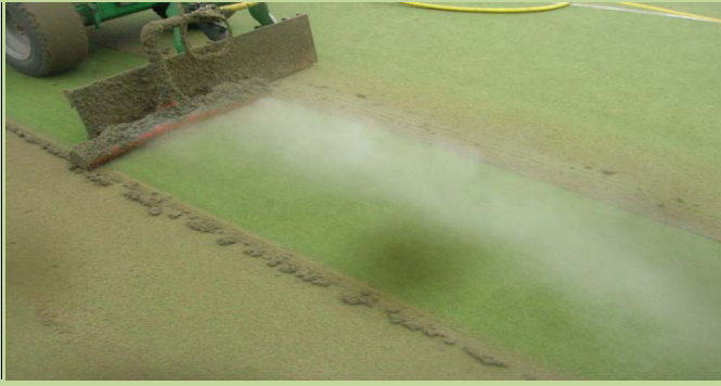
Rejuvination unit using compressed air to extract contaminated infill
