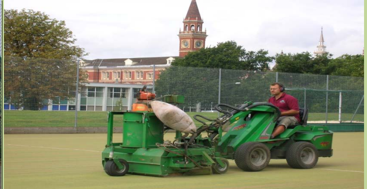
Astro turf pitch cleaning decompacting infill and removing contamination
