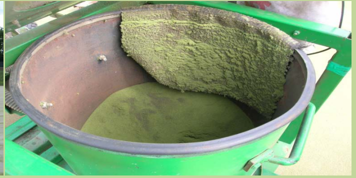
Contamination that has been extracted from astro turf pitch infill
